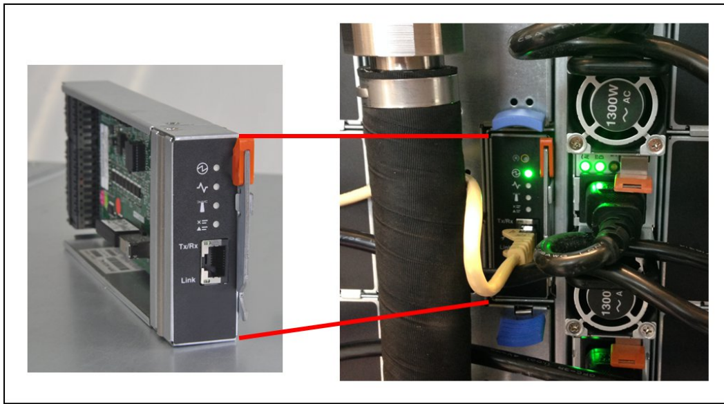
Figure 11. Fan and Power Controller
